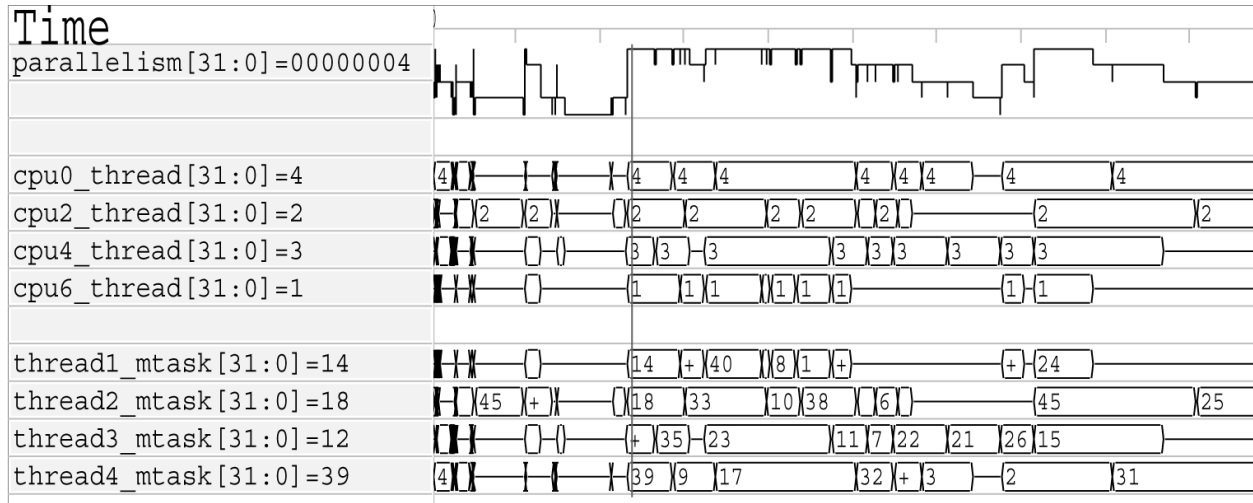
Fig. 6.1: Example verilator_gantt output, as viewed with GTKWave.
