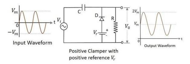
During the positive half cycle, the reference voltage is applied through the diode at the output and as the input voltage increases, the cathode voltage of the diode increase with respect to the anode voltage and hence it stops conducting. During the negative half cycle, the diode gets forward biased and starts conducting. The voltage across the capacitor and the reference voltage together maintain the output voltage level.
