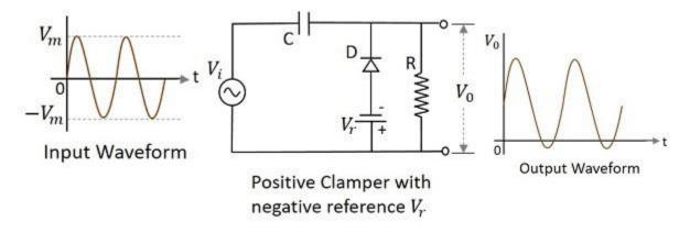
During the positive half cycle, the voltage across the capacitor and the reference voltage together maintain the output voltage level. During the negative half-cycle, the diode conducts when the cathode voltage gets less than the anode voltage. These changes make the output voltage as shown in the above figure.
