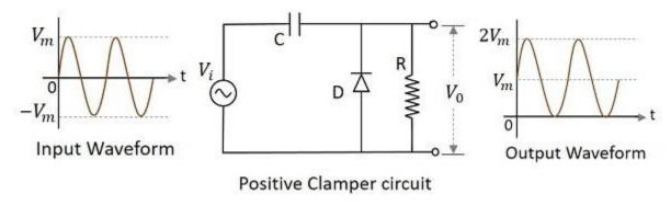
Initially when the input is given, the capacitor is not yet charged and the diode is reverse biased. The output is not considered at this point of time. During the negative half cycle, at the peak value, the capacitor gets charged with negative on one plate and positive on the other. The capacitor is now charged to its peak value  $V_mV_m$ . The diode is forward biased and conducts heavily.
