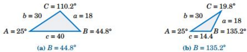
Figure 2.2: To solve the triangle when 2 sides and one opposite angle is given
