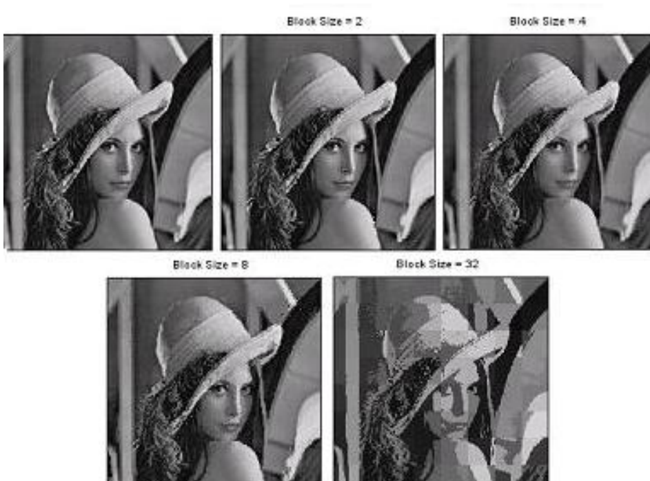
Figure 9.1: Program performs Block Truncation Coding
