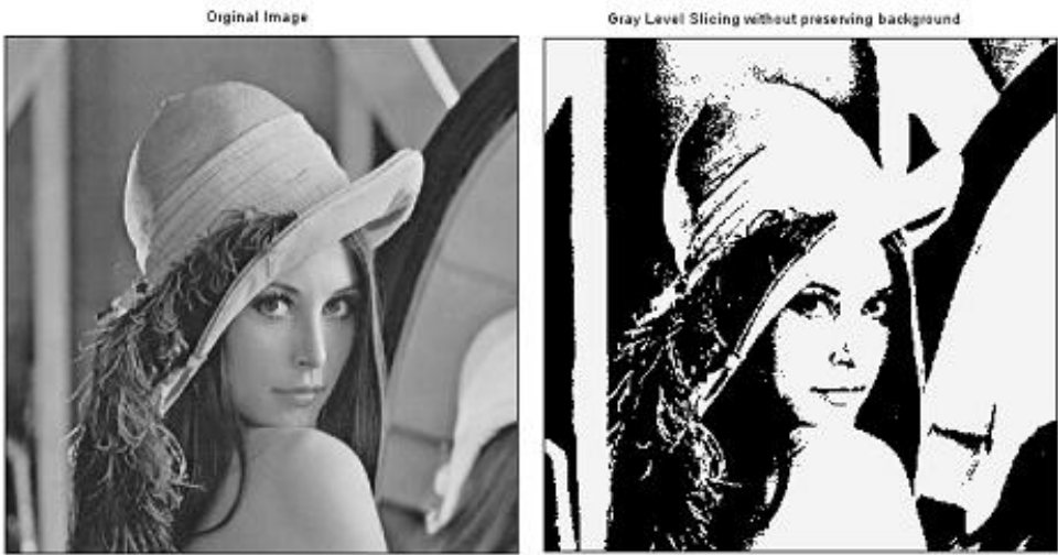
Figure 5.6: Program performs gray level slicing without background
