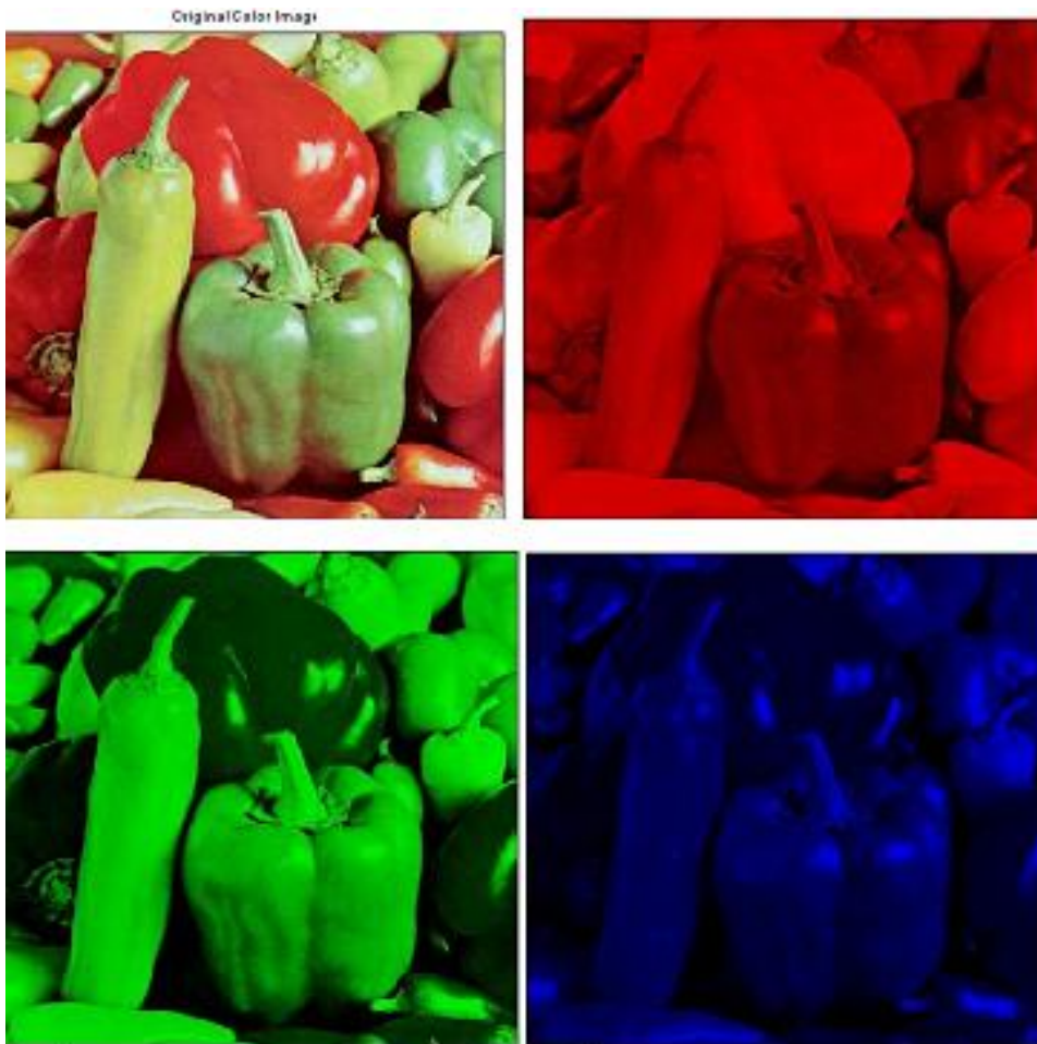
Figure 11.1: Read an RGB image and extract the three colour components red green blue
