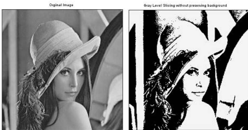
Figure 5.6: Program performs gray level slicing without background
